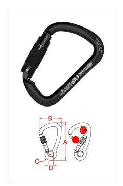
Light alloy carabiner with Auto Block sleeve. The X-Large is designed to offer a wide gate opening and a high tensile strength. The particular D shape prevents the rotation of the carabiner and allows to distribute the load along the major axis.
